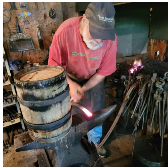
Blacksmith Rob Lyon fabricating iron hoops for the wellsweep bucket.
